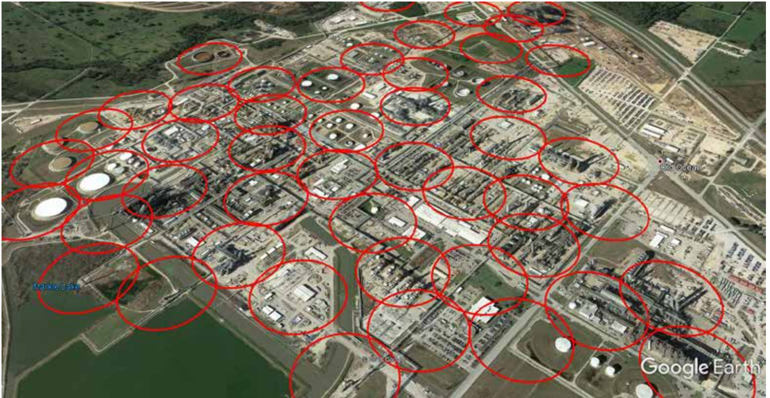
CPCHEM Sweeney TX reference. Each red circle represents one device with a coverage radius of 120 m each.
